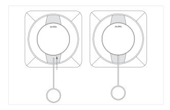
3 Hold the opening pin in position and turn the pin with the housing (shown as a gray area in the sketch) counterclockwise by approx. 10°. The operating panel is <u>not</u> rotated during this process.
