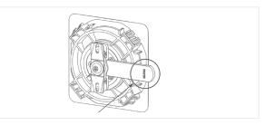
2 If the electronic lock is installed in the European Economic Community (EU and EFTA), the enclosed type plate must be clearly visible, legible and permanently affixed to the cam (on the back of the door). Otherwise the product does not comply with the safety standard of the RED (Radio Equipment Directive).
